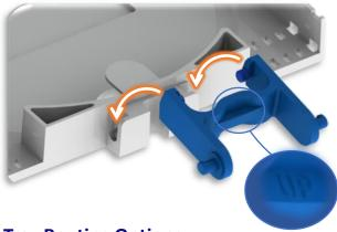
**Step 2** With the hinge attached to the tray, select the next available opening on the tray tower and snap hinge pins into the desired holes. Use the grooves to help align hinge pins.
